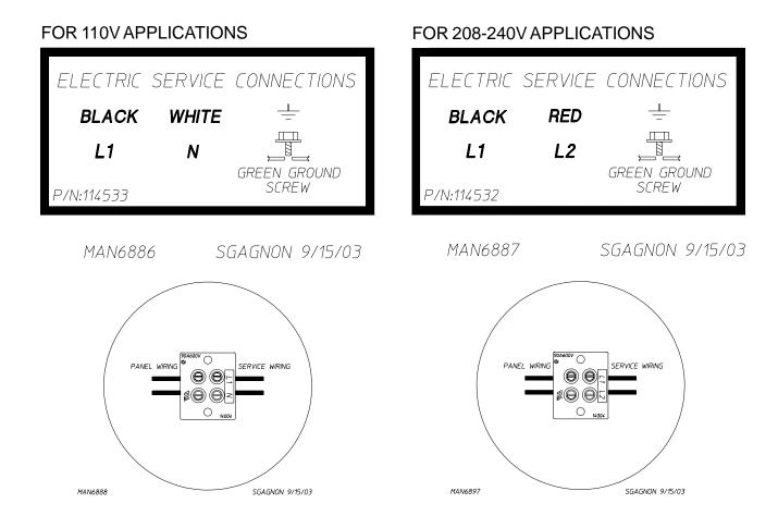
A ground lug is provided in the rear electrical box to connect your service ground.
